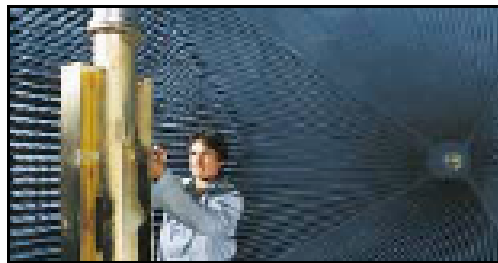
Full size antenna section undergoing a pressure test in one of two Andrew anechoic chambers dedicated to broadcast products.
